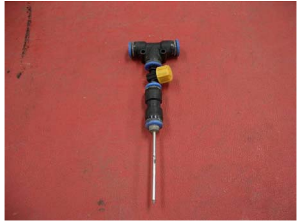
Injection needle with quick release connection and flow adjuster
